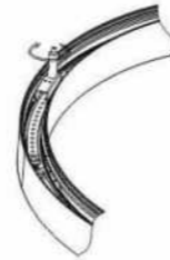
Step 06: Lock the U shape clip
