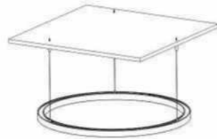
Step 06: Hang the circle by the steel wire
