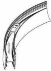
Step 01: Slide the U shape hanging clip into the profile
