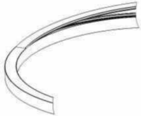
Step 03: Press the curved cover into the profile
