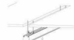
Step 07: Push the whole profile into the ceiling
