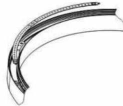
Step 05: Stick the led board inside the profile(up light)
