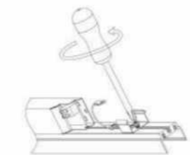
Step 04: Fix the internal clips and the driver
