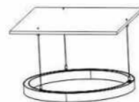
Step 09: Hang the circle by the steel wire
