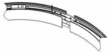
Step 02: Connecting the curved profile by connector
